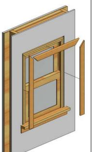
**b)** Remove interior stops from frame. If you plan to re-use interior stops, remove with caution.
