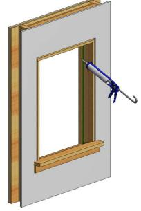
hung fixed only. Cut and apply the exterior stop cover. Miter the top corners of the cover and cut the sill end of the cover to match the sill angle. Nail all three exterior stop covers to the existing frame. Space the nails 3 inches from each end and 12 inches apart.
