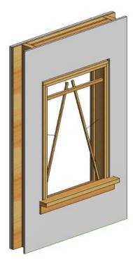
**e)** If applicable, remove parting stops from head and side jambs.
