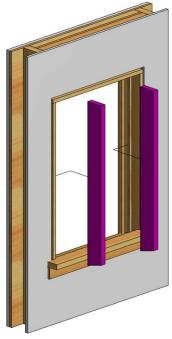
Remove existing balance system (Cut cords if necessary, detach pulleys).
