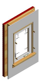
Appropriately shim the window to obtain a level and square window with uniform frame dimensions. \*Note\* Place a shim behind each installation screw hole and at the center on each side. Using the 2" pan head screws, screw the retro fit vinyl window to the existing frame. Install the provided hole caps. Removing the sash(s) may be required.
