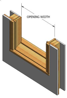
Measure the opening height of the existing frame at the left, right, and center of the frame (see left). Verify the replacement window frame height (from interior) is approximately 3/8" smaller than the existing frame height.
